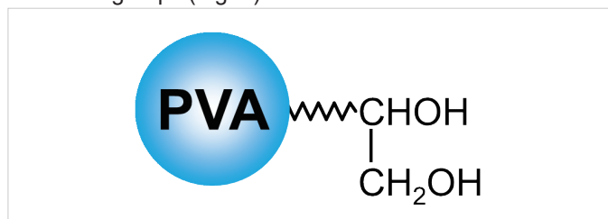
Fig. 1. Schematic diagram of VN-50 packing material
