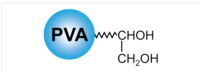
Fig. 1. Schematic diagram of VN-50 packing material
